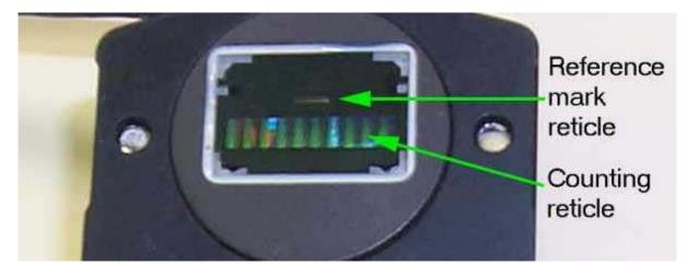
The signal for an optical encoder is obtained by the transmission and reception of light over the engraved markings on the encoder tape. The physical distance of the encoder head from the tape will affect how strong the received signal is due to focal length effects, as will be discussed later.
