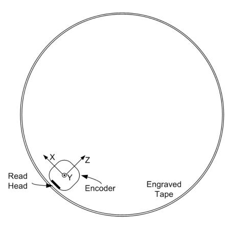
Here the important thing to note is that the direction of the x-axis is always in the clockwise direction when looking at the encoder ring from an outer side.
